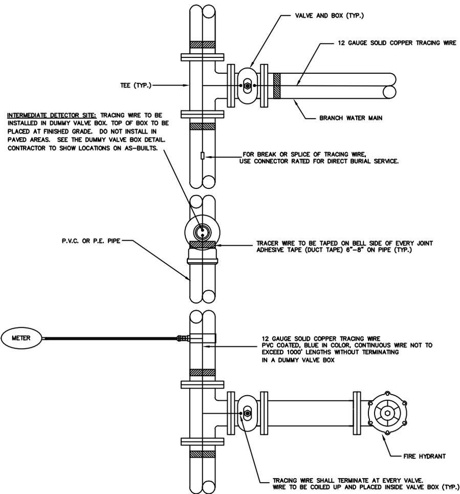
***TRACING WIRE INSTALLATION DETAIL***
